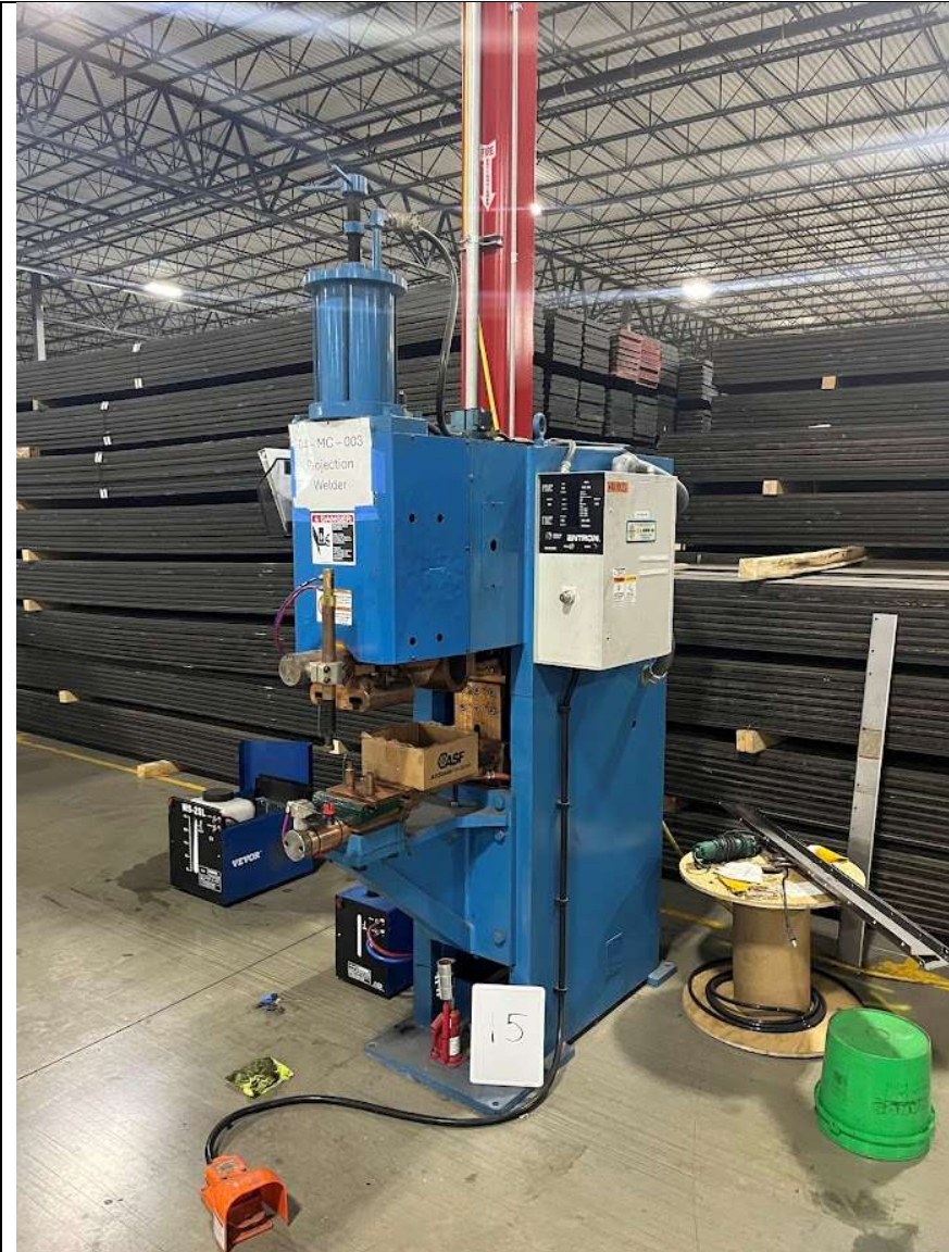
#15 – T.J Snow 100KVA Spot Welder
